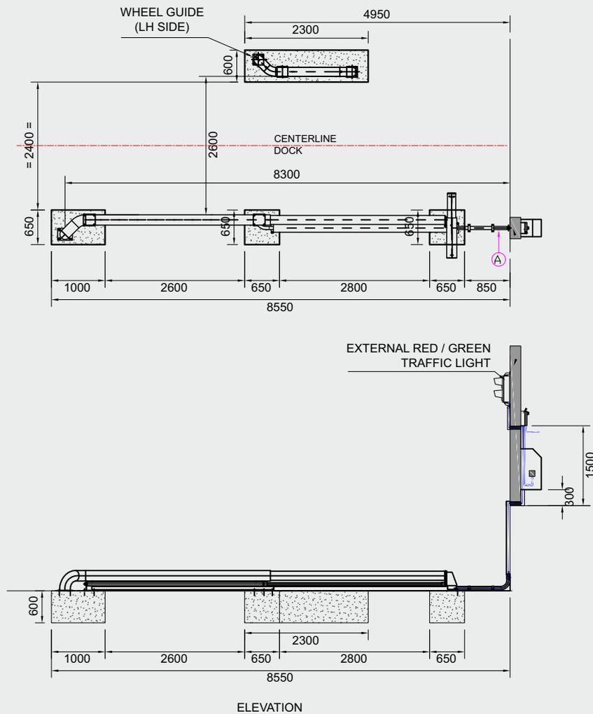
Gandhi Automations standard Motorised Wheel Block System is suitable for all types and size of trailer and trucks. Different types of wheel guides are available. These wheel guides will guide the vehicle for the perfect parking. This makes the Wheel Block a system which is extremely versatile. And it is easy to install on the ground.
